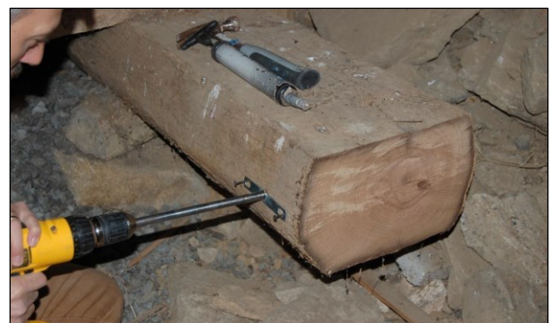
Detail of Bracing Joints at Swing Beam (left) and of Sample Extraction (below). Photo Credit: C. Cielo.
